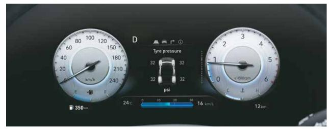
Tyre pressure monitoring system: Highline
